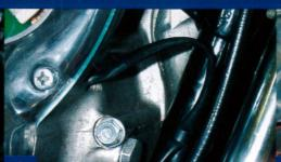
WHEN ROUTING THE STATOR WIRE TO THE ENGINE LEAVE A J SHAPED LOOP IN THE WIRE CLOSE TO THE ENGINE. THIS WILL STOP THE WIRE FROM BREAKING UNDER VIBRATION.
