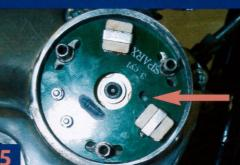
TURN THE ROTOR UNTIL YOU CAN SEE THE SCREW IN THE STATOR PLATE TIMING HOLE.
