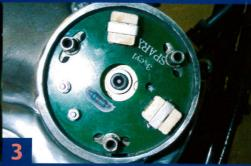
MOUNT THE STATOR PLATE WITH THE PILLAR BOLTS IN THE MIDDLE OF THE ADJUSTMENT SLOTS.
