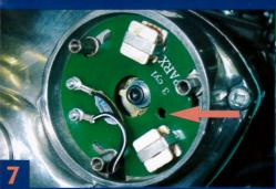
ROUTE THE STATOR PLATE WIRES VIA THE SHORTEST ROUTE (AVOIDING AC WIRES AS THESE CAN CAUSE INTERFERENCE) CUT TO LENGTH & USE SHIELDING SUPPLIED & CRIMP CONNECTORS SUPPLIED.
