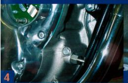
SET THE CRANKSHAFT IN THE B.T.D.C. POSITION.
