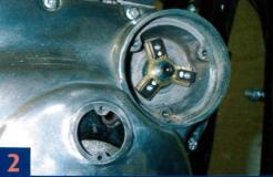
PLACE THE ROTOR INTO THE CAMSHAFT AND INSERT ALLEN BOLT AND LEAVE LOOSE SO YOU CAN ADJUST THE ROTOR POSITION.
