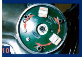
TURN THE STATOR PLATE ON ITS SLOTS UNTIL THE TIMING MARK ON THE ALTERNATOR ROTOR ALIGNS WITH THE POINTER ON THE COVER (USING A WHITE LINE ON THE ROTOR TIMING MARK WILL HELP).
