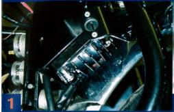
MOUNT THE IGNITER BOX IN A SUITABLE PLACE.
